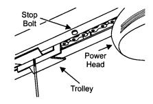
To confirm final OPEN travel adjustment, activate the opener to bring door to fully open position. The opener light should *not* be flashing.
